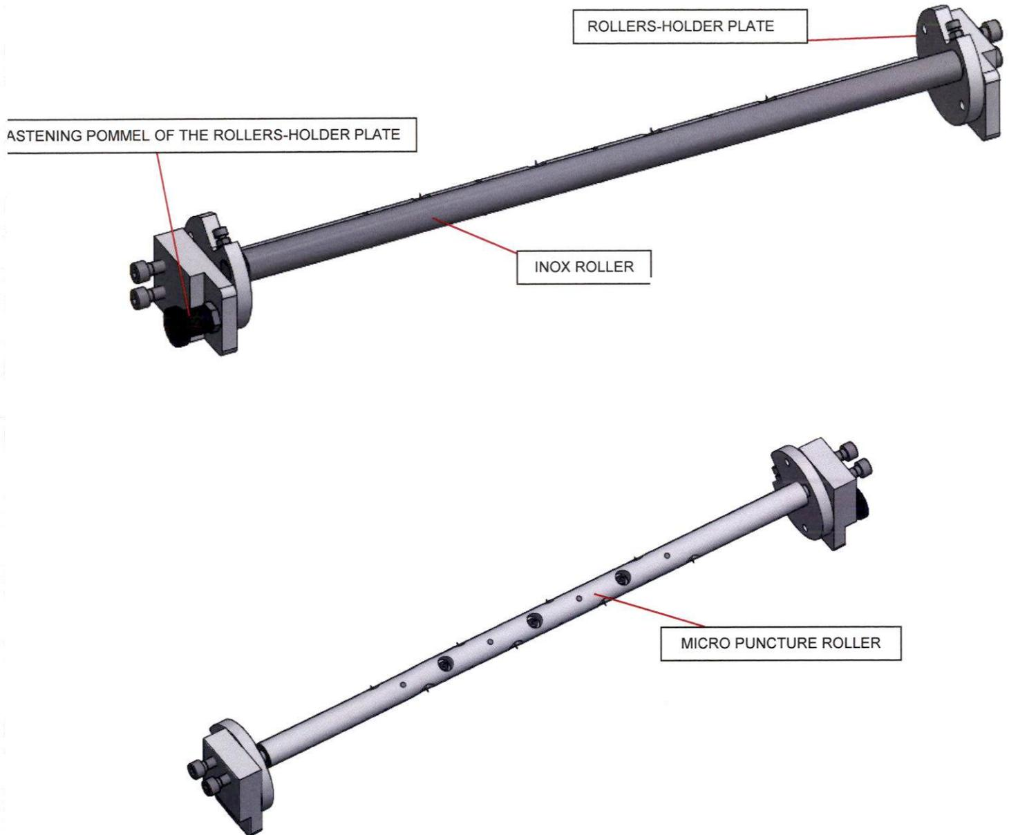
Fig. 10 Micro puncture system
